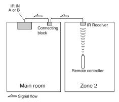
The miniplug cable from the connecting block should be connected to the AV receiver's IR IN A or B jack, as shown below. The IR IN A and B jacks are identical. Up to two IR receivers can be connected.
